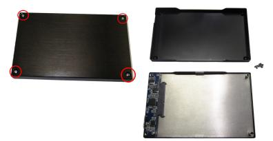
2. Place the 2.5" SATA drive into the half of the enclosure that contains the SATA connector, and slide the drive onto the SATA connector.
