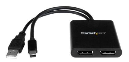
This MST hub lets you connect two DisplayPort monitors to your Mini DisplayPort computer. MST works on any Windows® device that supports DisplayPort 1.2, such as models of the Lenovo<sup>™</sup> Think Pad® and Microsoft® Surface<sup>™</sup>. When connected to earlier revisions of DisplayPort, such as DP 1.1 the MST hub acts as a video splitter. The MST hub is USB powered, so the only thing you'll need to operate the hub is your computer.
