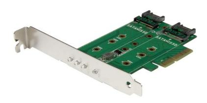
This 3-port M.2 SSD adapter card is one of the only cards that supports both PCIe and SATA-based M.2 SSDs (solid-state drives). It's a versatile way to expand the overall storage capacity of your desktop PC or server. Plus, because it supports a high-speed PCIe M.2 drive, you can increase the speed and performance of your computer.
